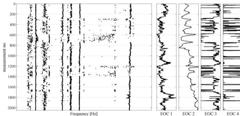
Figure 6. Long-term measurement and feature extraction of a rotating turbine.
