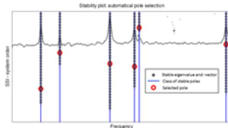
Figure 5. Stability diagram with automated pole selection.
