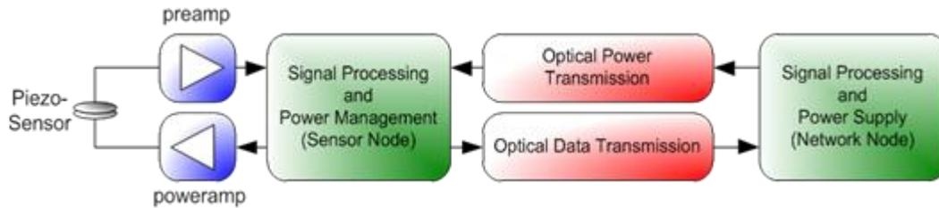
Figure 1. Optical power and data transmission.
