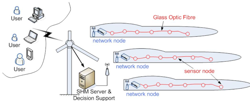
Figure 2. Sensor grid with nodes connected by optical fibres.
