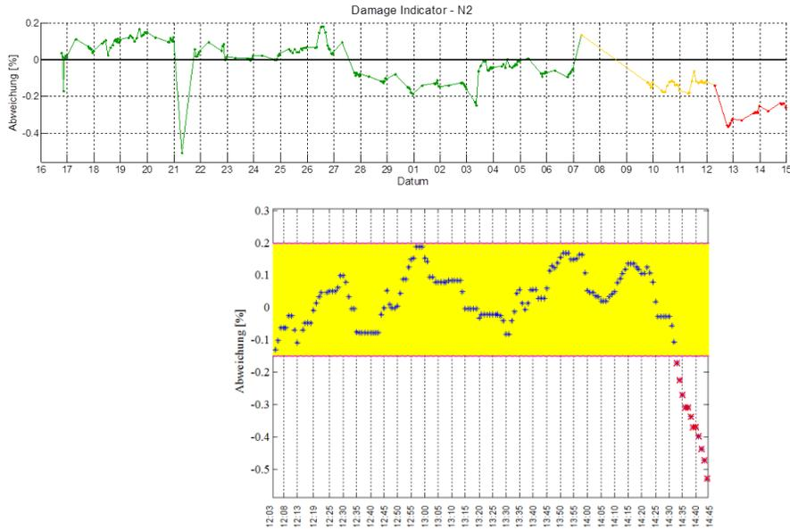
Figure 7. a, b: Objective of data processing is a clear indication of starting damage processes to allow for a stop right before failure.
