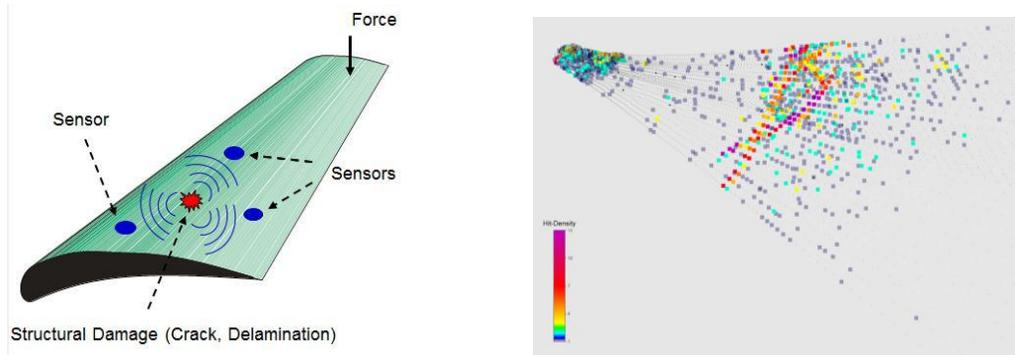
Figure 3. Functional principle of acoustic emission (left); result of a fatigue test of a blade (right).
