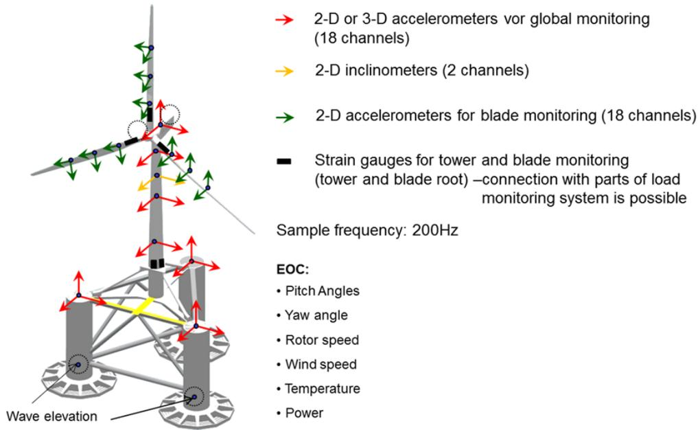
Figure 8. Instrumentation plan of HiPRwind floater.
