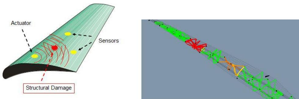
Figure 4. Functional principle of acousto ultrasonics (left); change of transfer-functions between emitter and receiver – red: no correlation between the emitted signal and the one received (right).
