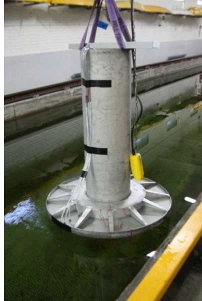
Figure 39 Damper and Column tank testing
